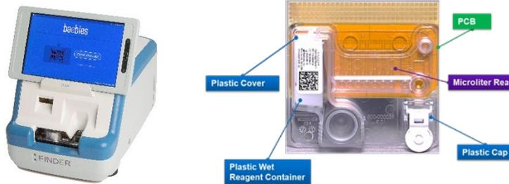
**Figure 1.** FINDER is a near-patient platform for rapid testing in a hospital or clinic setting. For molecular assays, FINDER can perform rapid PCR in ~5 minutes. All reagents are dried on a disposable cartridge and rehydrated during assay reactions. Sample dispensing, reagent mixing, and thermal cycling are automated on-cartridge. FINDER can accept multiple sample types, including saliva (for CMV), urine, or whole blood.
